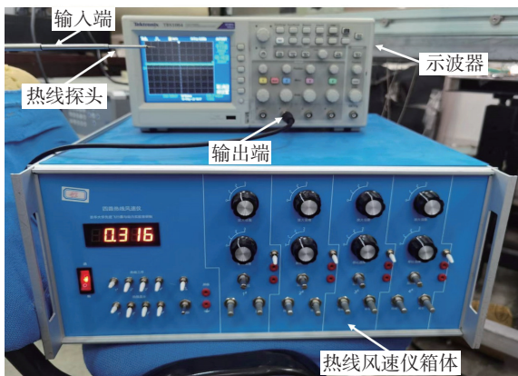
图2 热线风速仪测量系统 Fig. 2 Hot-wire anemometer measurement system
